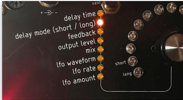
delay mode = **null** (VF-104 will not send midi data for delay mode)
